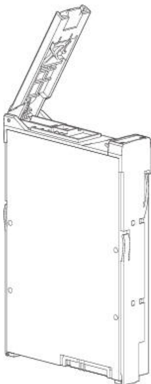
Figure 71. LFF drive carrier module in open position
