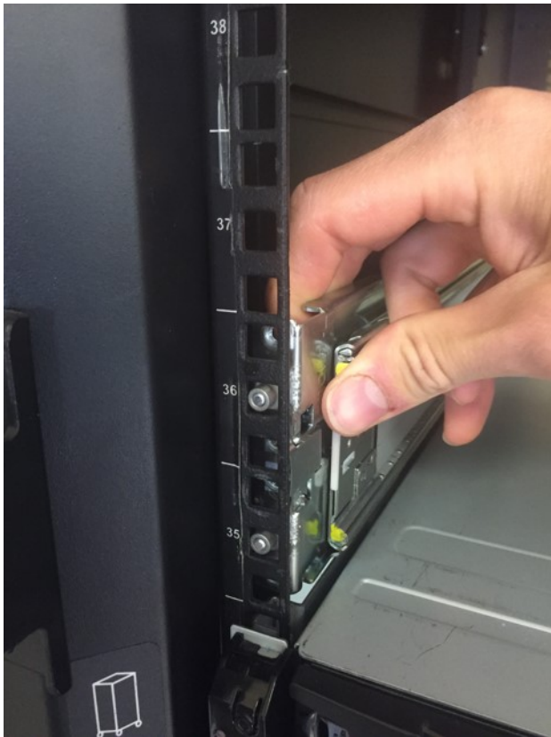
Figure 34. Front rack post attachment details
